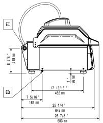
Electrical inlet (power) Electrical Outlet
